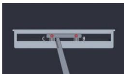
6. Use the supplied adjustment tool to rotate the gear under the point C until the gap is 0.4 mm. Then go back to the point A and fasten the fastening screw.
